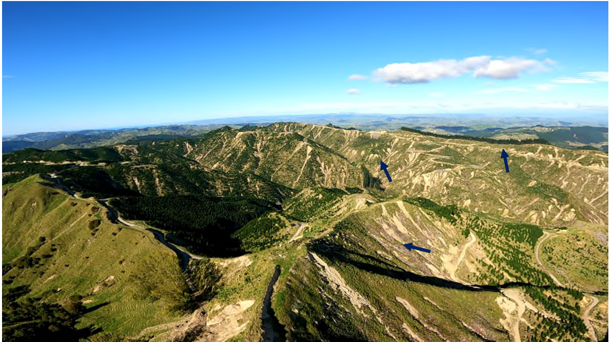
Infrastructure in the foreground has held up with minimal damage. However in the background there are many slumps / slips either onto the road or from the road (black arrows).
