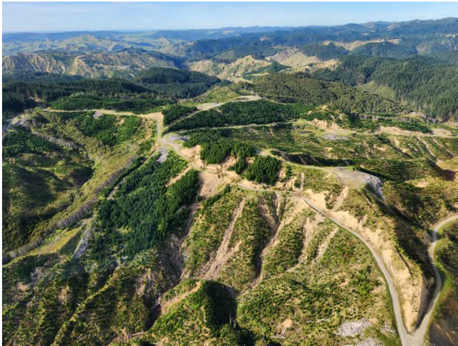
Pre-Labour weekend road and landing construction with many infrastructure triggered landslides evident, including from road and landing fill slopes
