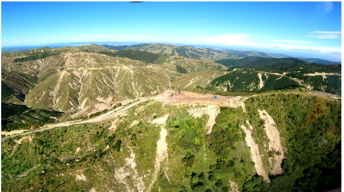
An example of a new-build landing that was in use by a cable yarding crew. Despite high construction standards and a relatively small footprint for such a large operation, there is still a slump right below the landing, a slip from the bench track on the left, and a slip most probably from the drainage as the road approaches the landing on the right.
